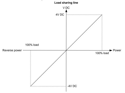
The active load sharing line is illustrated above, and the characteristics of the reactive load sharing line are equivalent to it.
